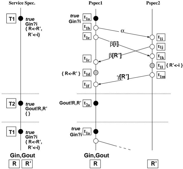
**Fig. 3.** Service specification and protocol Specification : timing charts
